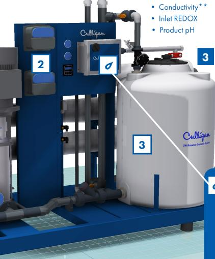
Extend the life of the membranes using the Integrated flushing tank option. Each time the unit shuts down or during alarm conditions the unit will flush the membranes with treated product water.
