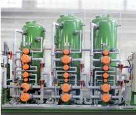
Skid-mounted demineralization plant with "polishing" column
