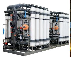
Ultrafiltration plant for reuse of wastewater
